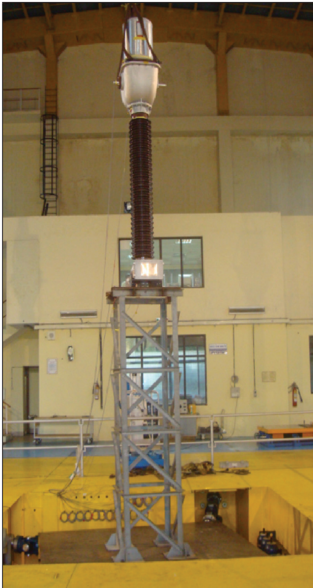
FIG.1 245 kV CURRENT TRANSFORMER WITH SUPPORT STRUCTURE MOUNTED ON TRI-AXIAL SHAKE-TABLE
