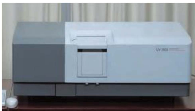
Figure 2. UV-Vis spectrometer used for transformer oil analysis.
