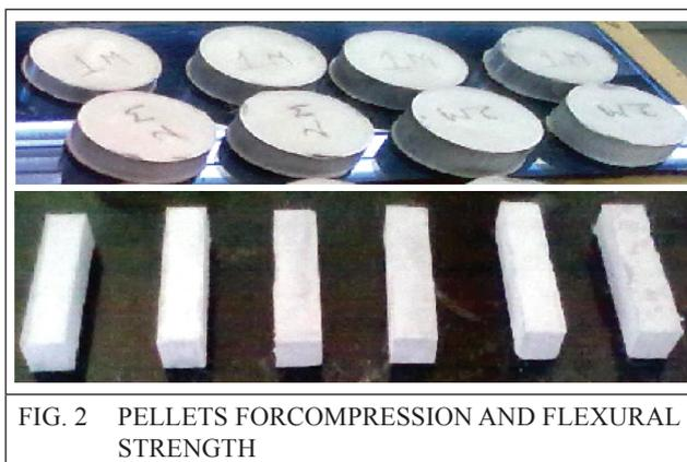
FIG. 2 PELLETS FOR COMPRESSION AND FLEXURAL STRENGTH
