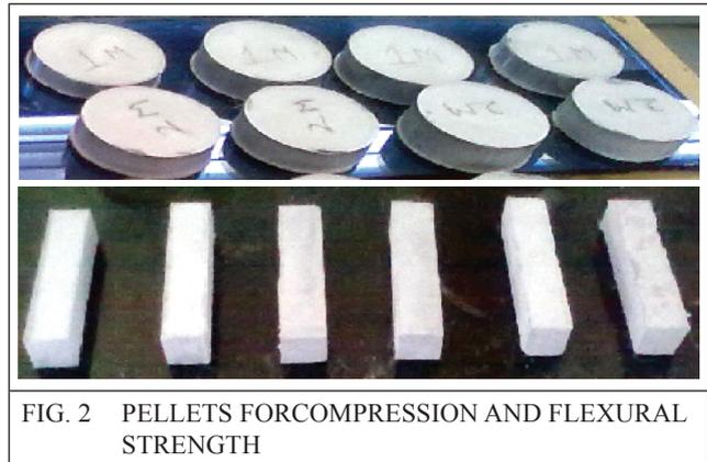
FIG. 2 PELLETS FOR COMPRESSION AND FLEXURAL STRENGTH
