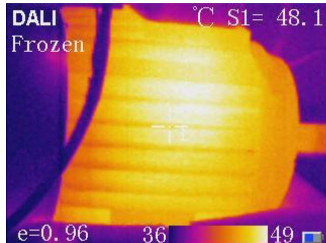
Figure 1. Thermal image of a running induction motor.
