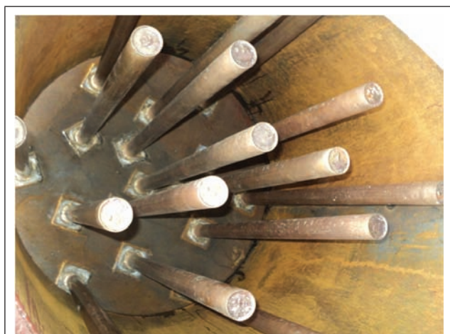
FIG. 4 CLOSE UP VIEW OF HEAT PIPES PLACED INSIDE CONDENSER
