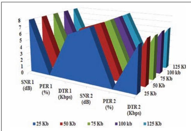
FIG. 7 DATA FILE TRANSMISSIONS ACROSS SECONDARY WINDINGS OF TWO 11 KV TRANSFORMERS
