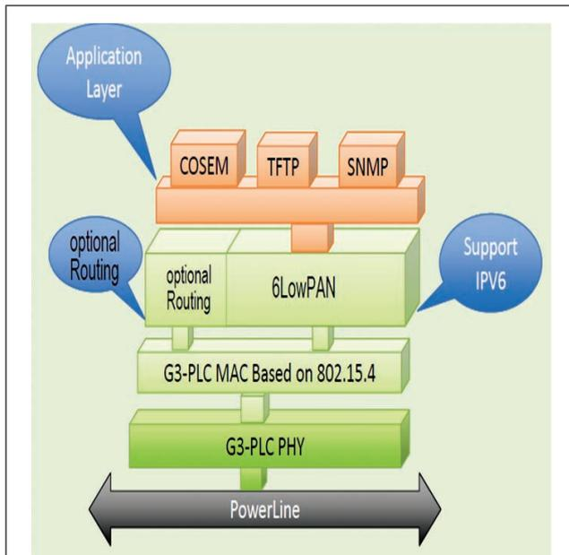
FIG. 1 G3-PLC TERMINAL PROTOCOL STACK
