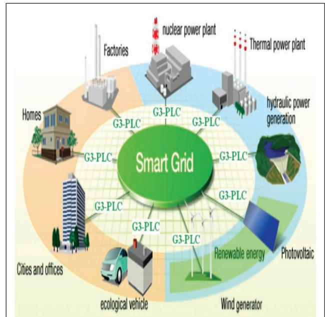
FIG. 2 A TYPICAL G3-PLC BASED SMART GRID INFRASTRUCTURE
