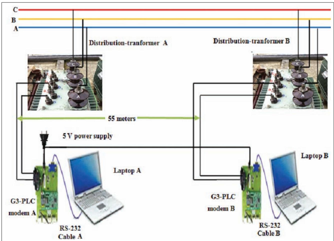
FIG. 5 EXPERIMENTAL SET-UP FOR G3-PLC PERFORMANCE ANALYSIS ACROSS SECONDARY WINDINGS OF TWO 11 KV DISTRIBUTION-TRANSFORMERS AT PANIPAT (HARYANA)
