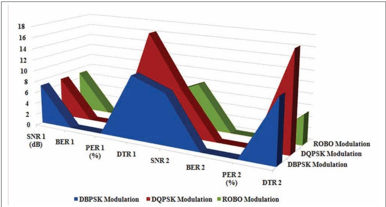
FIG. 6 PACKETS TRANSMISSIONS ACROSS SECONDARY WINDINGS OF TWO 11 KV TRANSFORMERS
