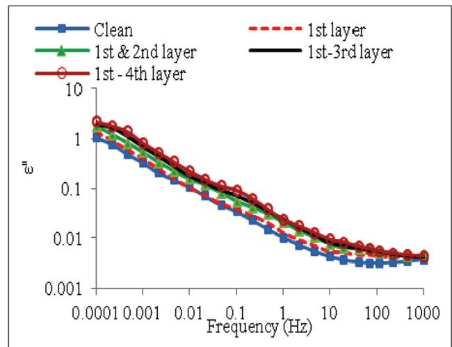
FIG. 9 VARIATION OF  $\epsilon''$  WITH FREQUENCY IN CLEAN AND  $\text{Cu}_2\text{S}$  CONTAMINATED PAPER AT 25° C.
