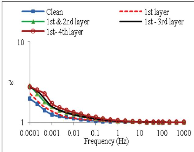
FIG. 6 VARIATION OF  $\epsilon'$  WITH FREQUENCY IN CLEAN AND  $\text{Cu}_2\text{S}$  CONTAMINATED PAPER AT 25° C.
