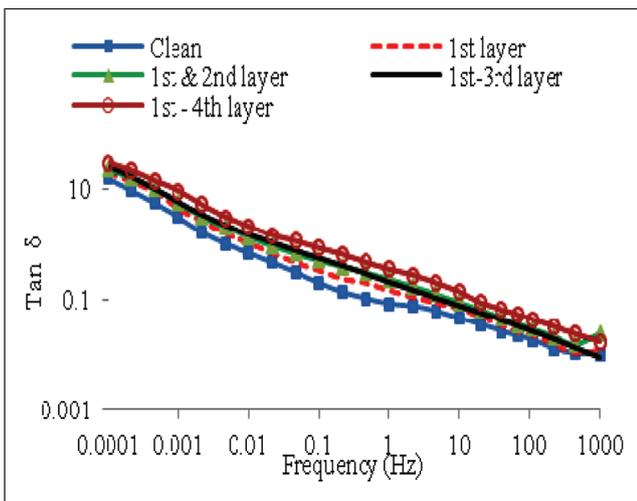
FIG. 4 VARIATION OF TAN Δ WITH FREQUENCY IN CLEAN AND CU<sub>2</sub>S CONTAMINATED PAPER AT 90° C
