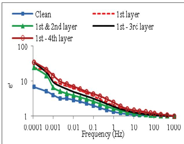
FIG. 8 VARIATION OF  $\epsilon'$  WITH FREQUENCY IN CLEAN AND  $\text{Cu}_2\text{S}$  CONTAMINATED PAPER AT 140° C.
