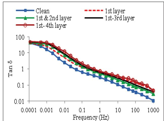
FIG. 5 VARIATION OF TAN Δ WITH FREQUENCY IN CLEAN AND CU<sub>2</sub>S CONTAMINATED PAPER AT 140° C
