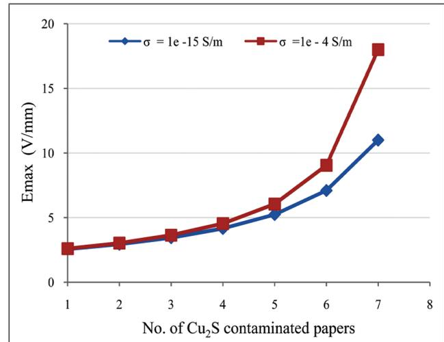
FIG. 2 VARIATION OF MAXIMUM ELECTRIC STRESS ON CLEAN PAPER LAYERS WITH NUMBER OF CU<sub>2</sub>S CONTAMINATED LAYERS
