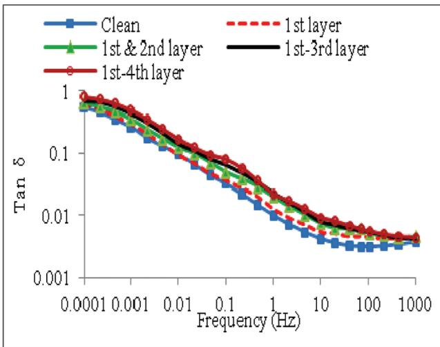
FIG. 3 VARIATION OF TAN Δ WITH FREQUENCY IN CLEAN AND CU<sub>2</sub>S CONTAMINATED PAPER AT 25° C.
