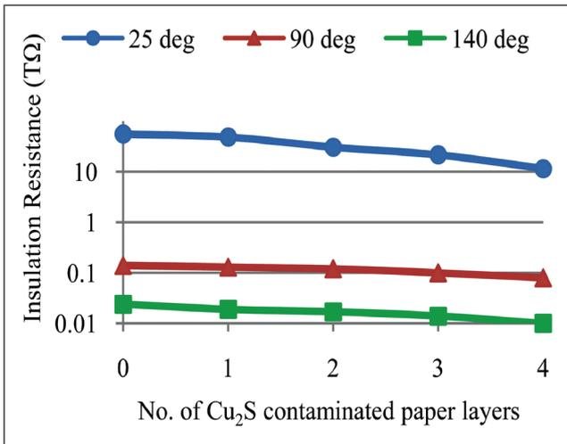
FIG.12 VARIATIONS OF INSULATION RESISTANCE FOR CLEAN AND  $Cu_2S$  CONTAMINATED PAPER AT  $25^\circ C$ ,  $90^\circ C$  AND  $140^\circ C$
