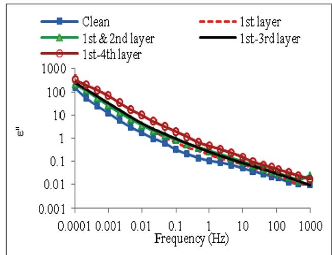
FIG. 10 VARIATION OF  $\epsilon''$  WITH FREQUENCY IN CLEAN AND  $\text{Cu}_2\text{S}$  CONTAMINATED PAPER AT 90° C.
