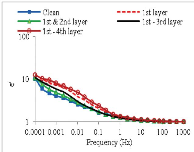
FIG. 7 VARIATION OF  $\epsilon'$  WITH FREQUENCY IN CLEAN AND  $\text{Cu}_2\text{S}$  CONTAMINATED PAPER AT 90° C.
