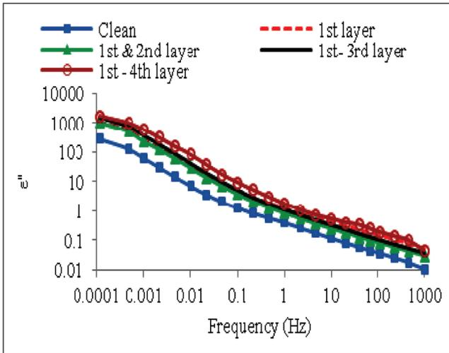
FIG. 11 VARIATION OF  $\epsilon''$  WITH FREQUENCY IN CLEAN AND  $Cu_2S$  CONTAMINATED PAPER AT  $140^\circ C$ .
