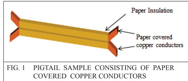
FIG. 1 PIGTAIL SAMPLE CONSISTING OF PAPER COVERED COPPER CONDUCTORS
