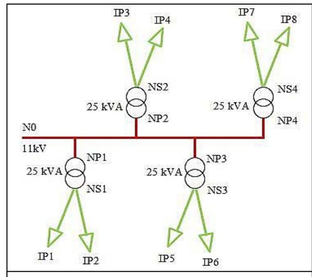
**Figure 2.** High voltage distribution system network.
