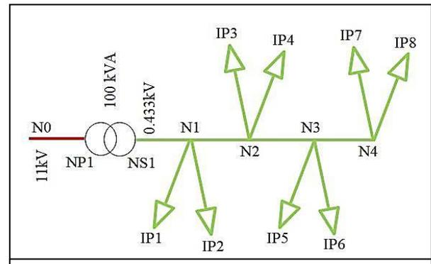
**Figure 1.** Low voltage distribution system network.
