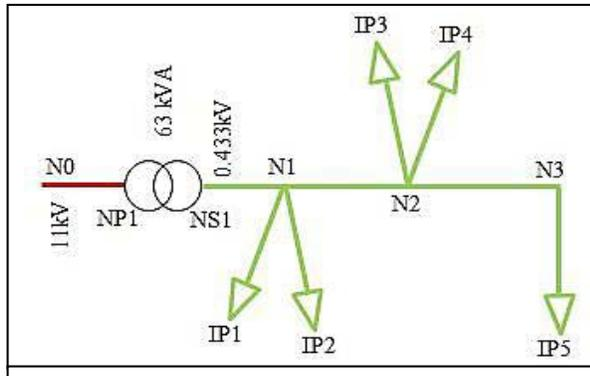
Figure 3. Low voltage distribution system network.
