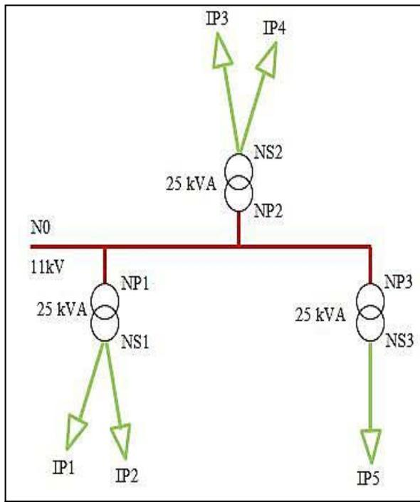
Figure 4. High voltage distribution system network.
