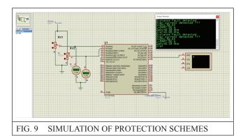
The simulated results of the protection scheme logic is shown above. In the simulation, the cutoff limits of a typical 400 kV feeder is considered as reference values. The controller is the integral part of the PDC unit and when it is interfaced with a GPS module, time-stamped measurements are fetched and manipulated.
