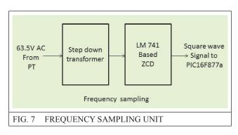
Zero crossing detector is used to convert sine wave or other signal into square-wave, the output should be low if the input is negative and high if the input if positive. A zero crossing detector literally detects the transition of a signal waveform from positive and negative, ideally providing a narrow pulse that coincides exactly with the zero voltage condition.
