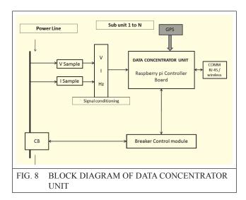
The time-stamped measurements from the data concentrator are simultaneously communicated to the master controller at the remote end and the substation controller at the local end. For master controller, wireless communication is deployed, while for local controller, wired communication is deployed. Thus, a two stage protection scheme is developed, so as to create a module with 100% reliability.
