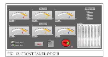
The picture illustrated above represents the front panel of the GUI. The front panel is crafted with analog and digital meters to cast the
