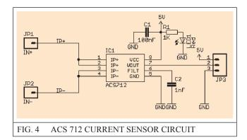
The device consists of accurate, low-offset, linear hall sensor circuit with a copper conduction path located near the surface of the die. Applied current flowing through this copper conduction path generates a magnetic field which is sensed by the integrated hall IC and converted into a proportional voltage.
