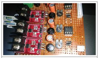
FIG. 6 HARDWARE CIRCUITRY OF THE CURRENT SAMPLING UNIT
