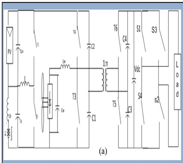
Figure 4. Converter configuration of whole system.
