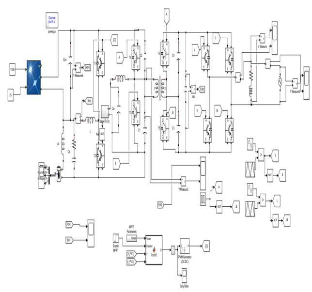
**Figure 8.** MATLAB model of PV with MPPT and Wind sources integration.
