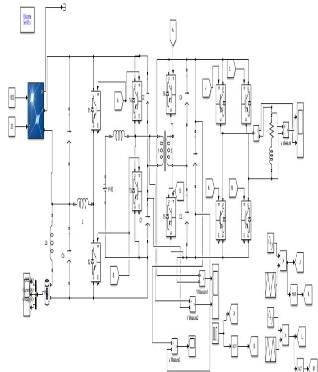
**Figure 6.** MATLAB model of PV and dc voltage integration.
