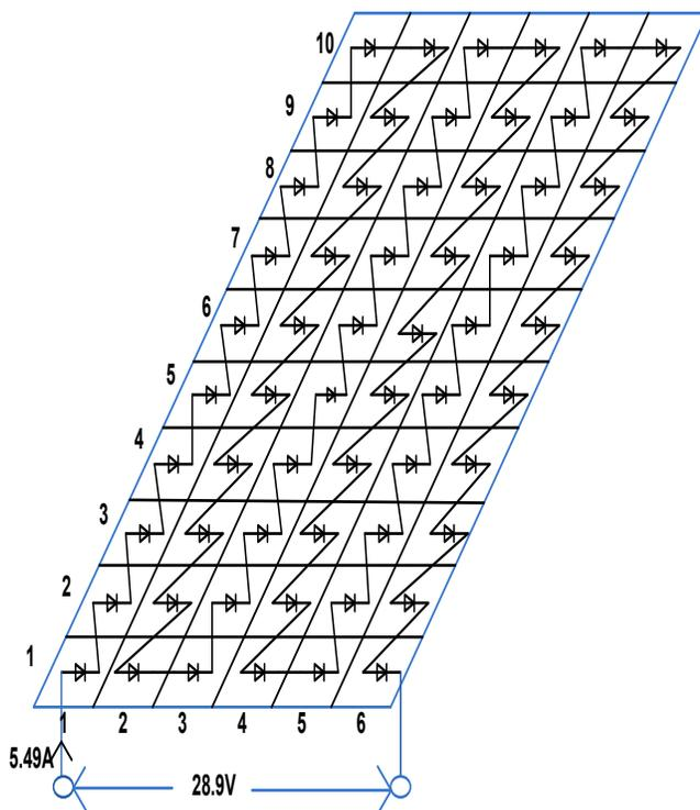
**Figure 1.** A photo-voltaic cell stack.
