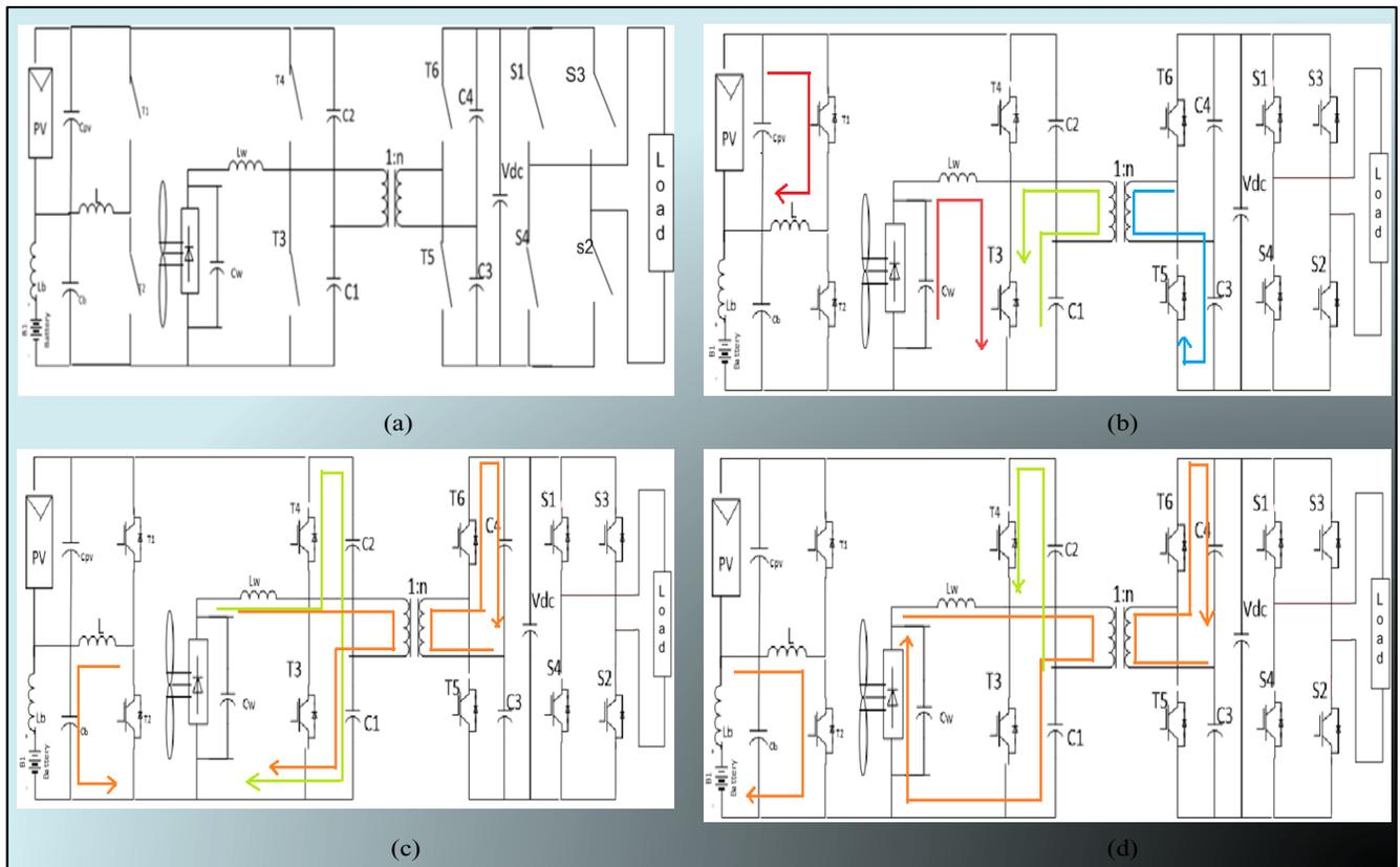
**Figure 3.** Various operating modes of the multi-input transformer-coupled bidirectional dc–dc converter. **(a)** Proposed converter configuration. **(b)** Operation when switch T3 is turned ON. **(c)** Operation when switch T4 is ON, charging the capacitor bank. **(d)** Operation when switch is T 4 ON, capacitor C2 discharging.
