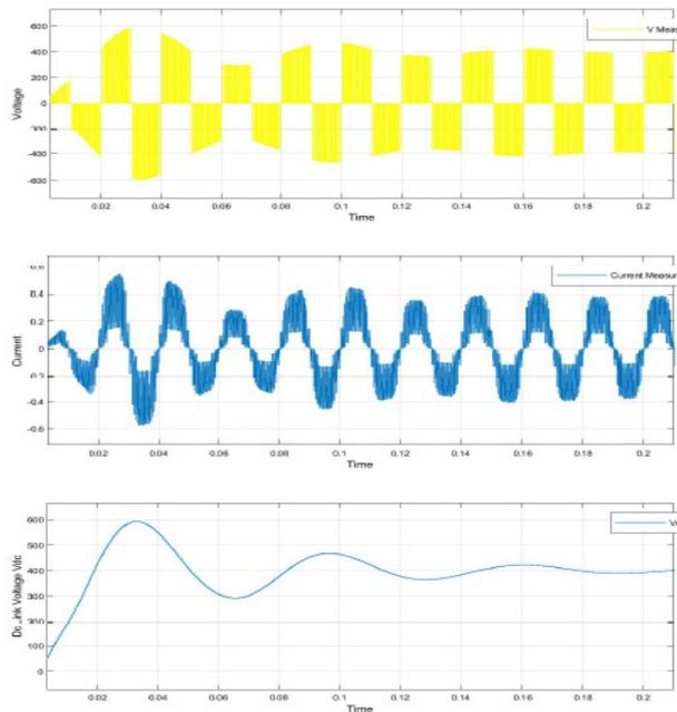
**Figure 9.** Output voltages, output current and DC link voltage waveforms of PV with MPPT and wind integration.
