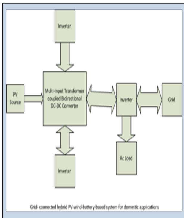
Figure 5. Block diagram of whole system.
