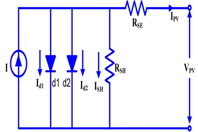
**Figure 2.** Equivalent circuit of the two diode model of PV cell.
