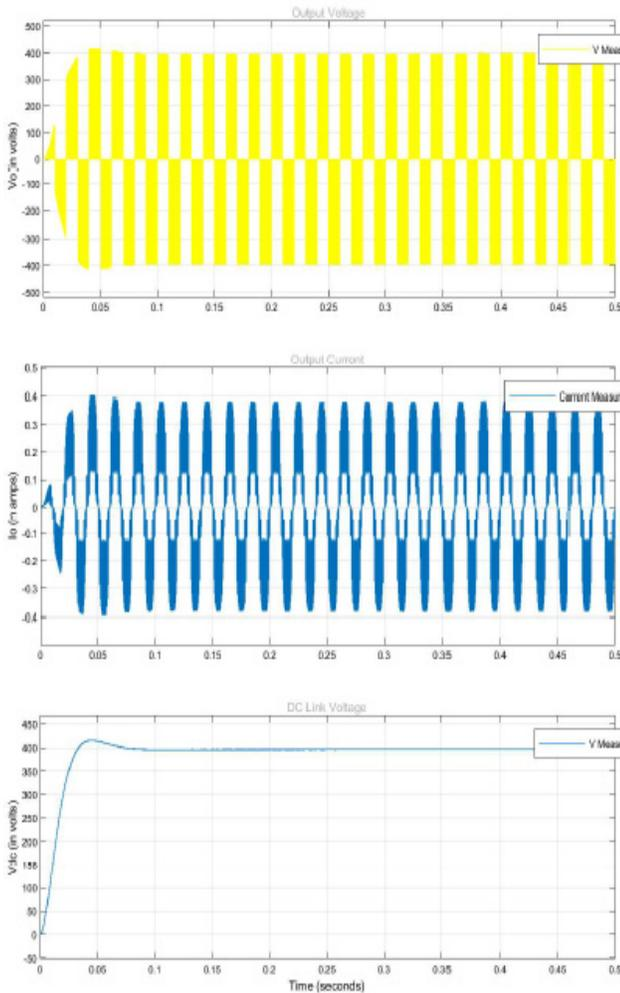
**Figure 7.** Output voltage, Output current and DC link voltage waveforms.
