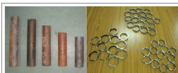
FIG. 1. BOILER TUBE SAMPLES AND MACHINED RING TUBE SPECIMENS
