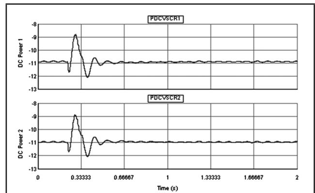
FIG 7 (A). POWER THROUGH DC LINE 1 & 2
