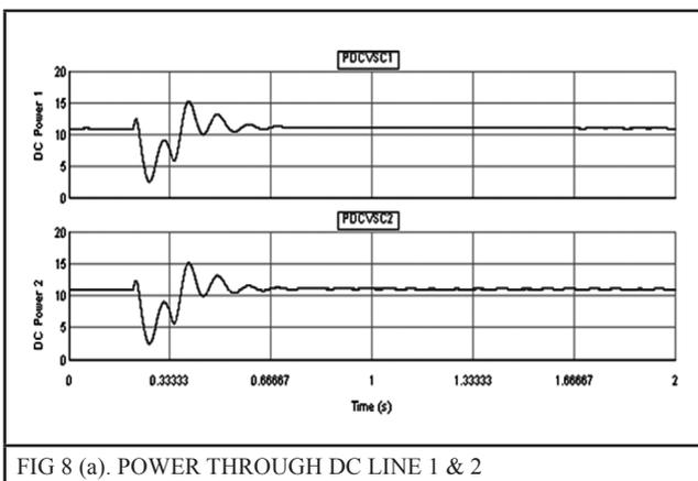
In this scenario, three phase to ground fault is applied at receiving end for a duration of 100 ms. The plots of DC line power are shown in Figure 8(a).
