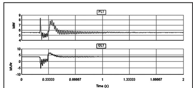
FIG 7 (C). ACTIVE AND REACTIVE POWER OF MOTOR M1 & M2
