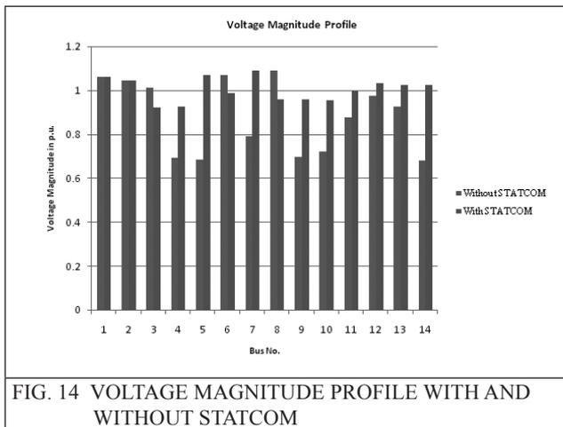
FIG. 14 VOLTAGE MAGNITUDE PROFILE WITH AND WITHOUT STATCOM
