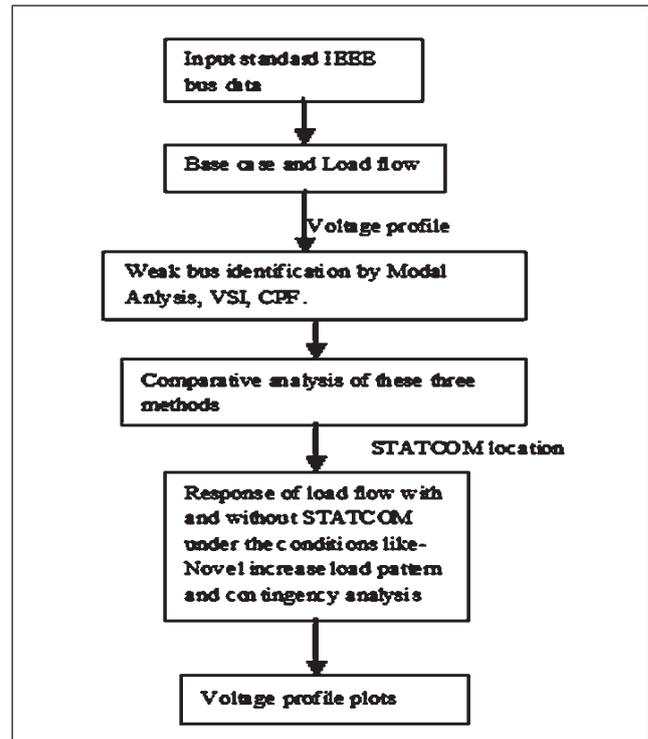
FIG. 6 OUTLINE FOR SYSTEMATIC METHODOLOGY FOR PLACEMENT OF STATCOM
