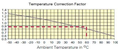
**Figure 1.** This Curve shows the influence of the ambient temperature on the fuse link's current carrying capability.
