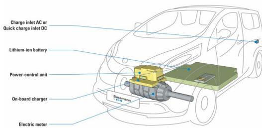
Typical fuse applications in an electric vehicle
