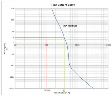
**Figure 6.** Time current curve.
