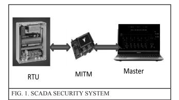
The CDAC - SCADA system as shown in Figure 1, comprises of Remote Terminal Unit(RTU), Man In The Middle(MITM) and System Operator console(Master).
