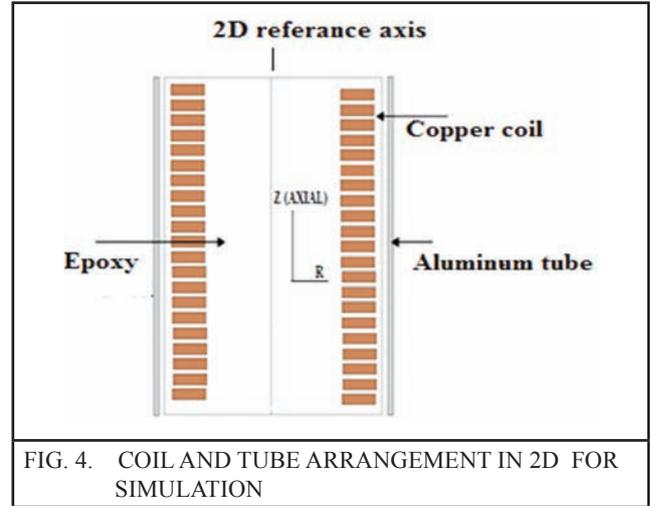
FIG. 4. COIL AND TUBE ARRANGEMENT IN 2D FOR SIMULATION
