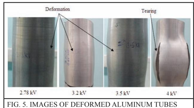
FIG. 5. IMAGES OF DEFORMED ALUMINUM TUBES
