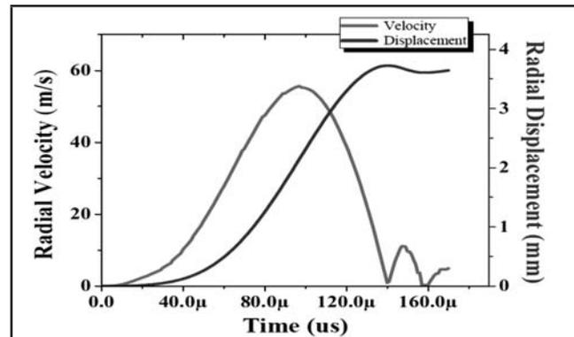
FIG. 7. RADIAL VELOCITY AND DISPLACEMENT OF TUBE WITH TIME AT 2.45 KJ
