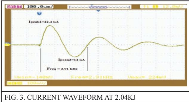
FIG. 3. CURRENT WAVEFORM AT 2.04KJ
