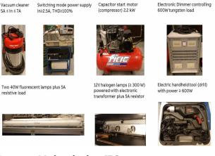
Figure 6. Masking loads in IEC62606.
