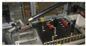
Figure 7. Parallel arc cable cutting test.
