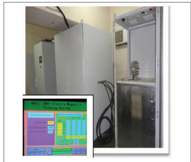
FIG 1. ELECTROMAGNETIC MANUFACTURING MACHINE DEVELOPED AT ACCELERATOR AND PULSE POWER DIVISION (APPD), BHABHA ATOMICRESEARCHCENTRE (BARC)
