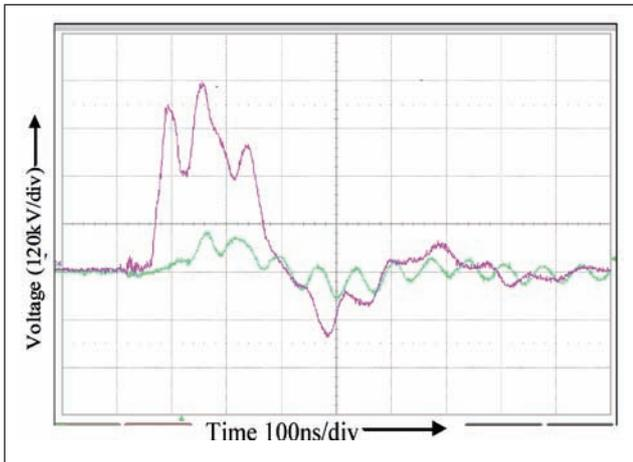
FIG. 9 MEASURED OUTPUT VOLTAGE WAVEFORM (PINK) OF THE 22-STAGE MARX GENERATOR WITH CONICAL ENCLOSURE
