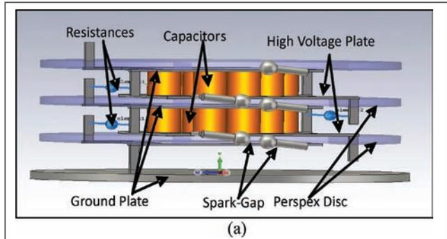
FIG. 3 (A) FIRST TWO STAGES OF MARX GENERATOR (YELLOW-CAPACITOR, BLUE- CHARGING AND GROUND RESISTOR)
