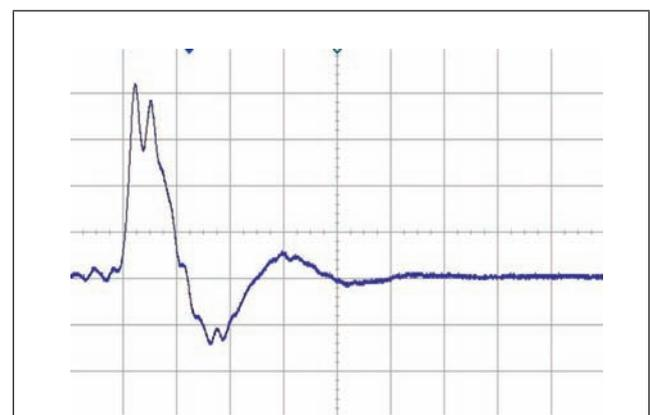
FIG. 8. MEASURED OUTPUT VOLTAGE WAVEFORM OF THE 22-STAGE MARX GENERATOR WITH CYLINDRICAL ENCLOSURE.
