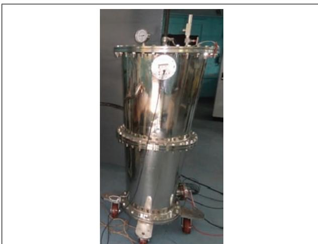
FIG. 7. 22-STAGEMARX GENERATOR WITH CONICAL ENCLOSURE
