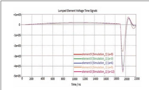
FIG. 6. SIMULATED OUTPUT WAVEFORM OF MARX GENERATOR ON CST MICROWAVE STUDIO WITH TOP RADIUS FROM 20 TO 32CM (5 SAMPLES) WITH LOAD RESISTANCE OF 100Ω
