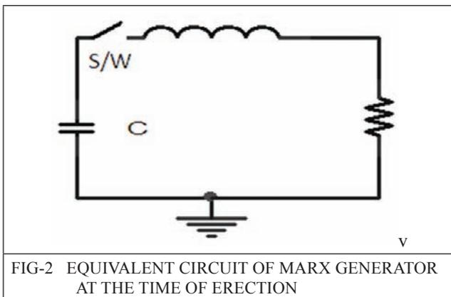
The impedance of the system is given by equation
