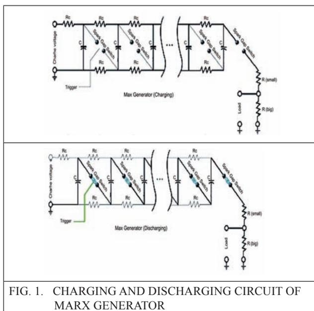
In this paper, the effects of stray capacitance and inductance which are related to the geometry of the enclosure of the Marx Generator have been studied. Efforts have been made to quantify these effects by using conical structure as the enclosure for Marx Generator. These effects have been observed in simulation of 22 stages 450 kV Marx Generator and are validated experimentally.
