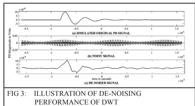
FIG 3: ILLUSTRATION OF DE-NOISING PERFORMANCE OF DWT
