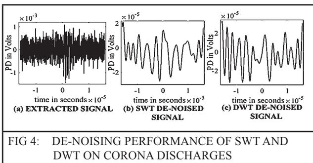
FIG 4: DE-NOISING PERFORMANCE OF SWT AND DWT ON CORONA DISCHARGES
