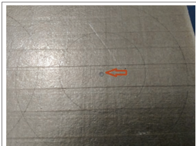
FIG. 1. SAMPLE USED FOR PD MEASUREMENT SHOWING VOID ON THE SURFACE
