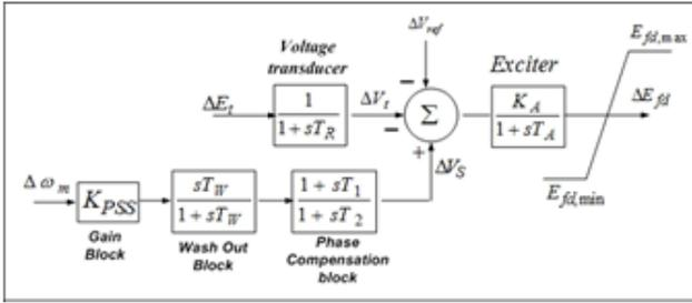
Figure 2. Simplified block diagram for proposed PSS
