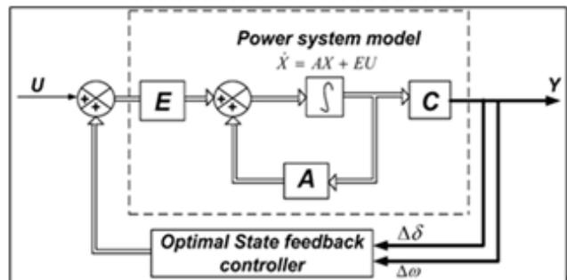
Figure 5. Block diagram representation of Optimal state feedback controller
