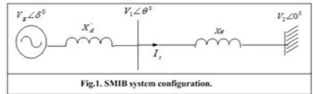
Figure 1. SMIB system configuration.
