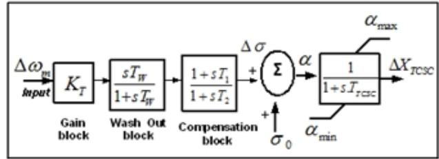
Figure 4. Simplified block diagram for proposed TCSC controller
