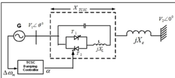
Figure 3. SMIB system with TCSC
