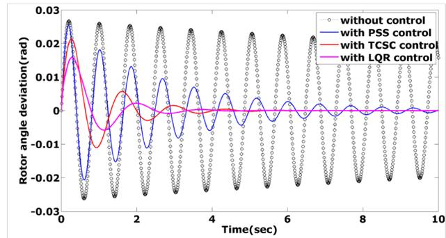
**Figure 8.** Rotor angle response of SMIB system
