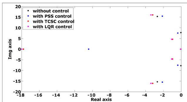
**Figure 7.** Eigenvalues for the SMIB bus at nominal load
