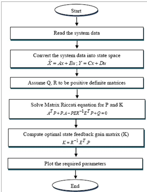
Figure 6. Flow Chart for the design of OSFC
