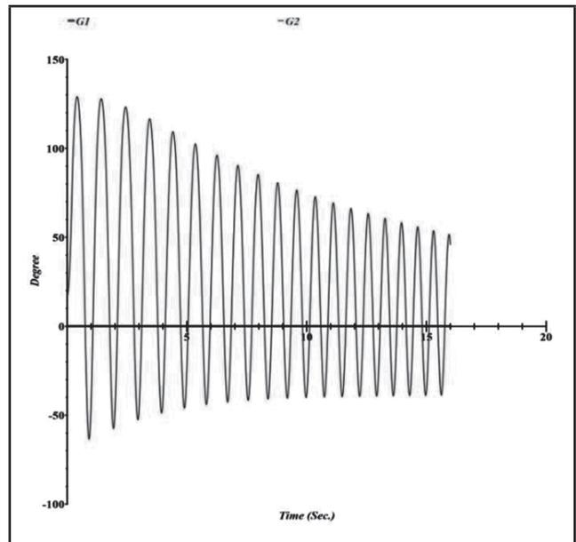
FIG.6. SYSTEM RESPONSE OF THE 9-BUS SYSTEM WITH WIND POWER: RELATIVE POWER ANGLE OF G1 AND G2 FOR THE SYSTEM WITH FCT=0.2S.
