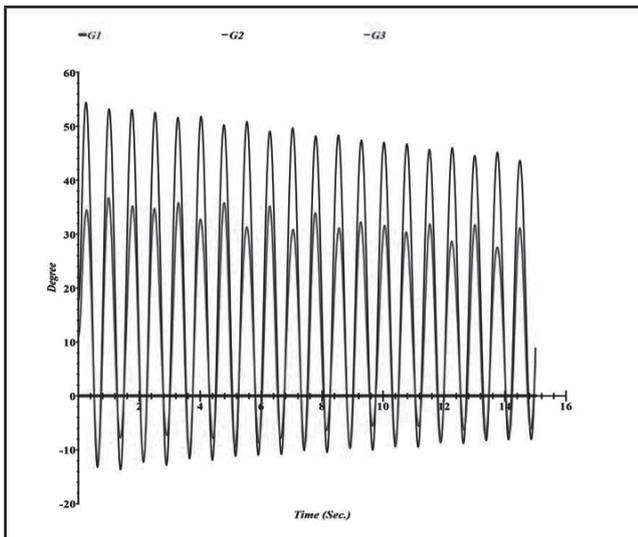
FIG.2. SYSTEM RESPONSE OF THE 9-BUS SYSTEM WITHOUT WIND POWER: RELATIVE POWER ANGLE OF G1, G2 AND G3 FOR THE SYSTEM WITH FCT=0.1S.
