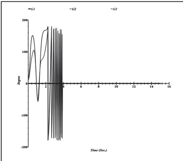
FIG.4. SYSTEM RESPONSE OF THE 9-BUS SYSTEM WITHOUT WIND POWER: RELATIVE POWER ANGLE OF G1, G2 AND G3 FOR THE SYSTEM WITH FCT=0.223S.
