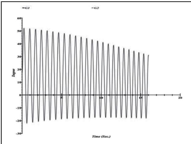
FIG.5. SYSTEM RESPONSE OF THE 9-BUS SYSTEM WITH WIND POWER: RELATIVE POWER ANGLE OF G1 AND G2 FOR THE SYSTEM WITH FCT=0.1S.
