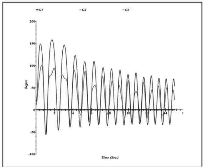
FIG.3. SYSTEM RESPONSE OF THE 9-BUS SYSTEM WITHOUT WIND POWER: RELATIVE POWER ANGLE OF G1, G2 AND G3 FOR THE SYSTEM WITH FCT=0.222S.
