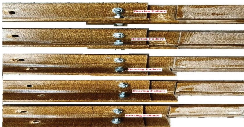
Figure 2. Angle-to-angle bolt connection tested specimens.
