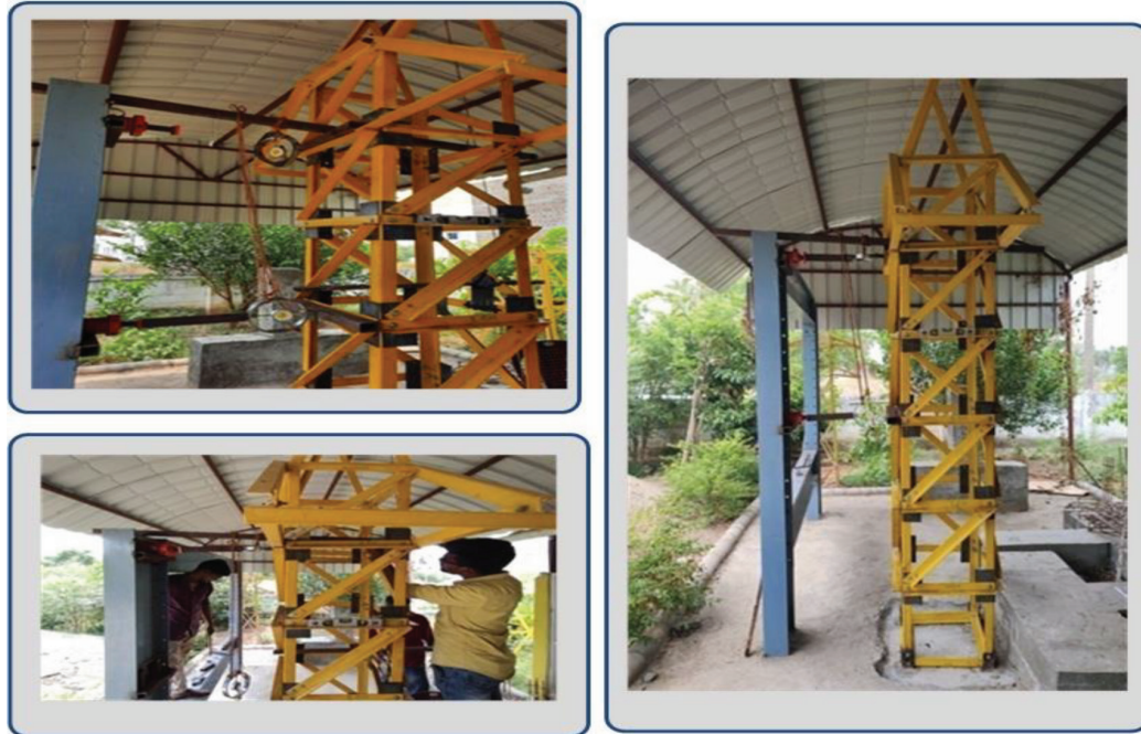
Figure 5. Testing on the GFRP transmission tower.
