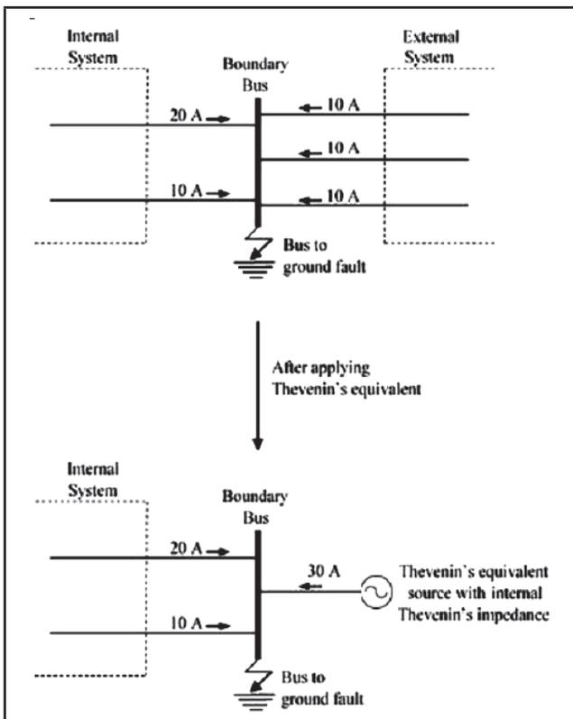
FIG. 3 THEVENIN'S EQUIVALENT AT BOUNDARY BUSES SUPPLYING THE SAME SHORT CIRCUIT CURRENT AS THE EXTERNAL SYSTEM
