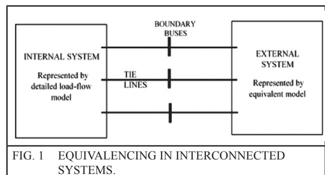
FIG. 1 EQUIVALENCING IN INTERCONNECTED SYSTEMS.
