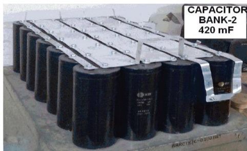
Figure 4. Additional capacitor bank of 420 mF.
