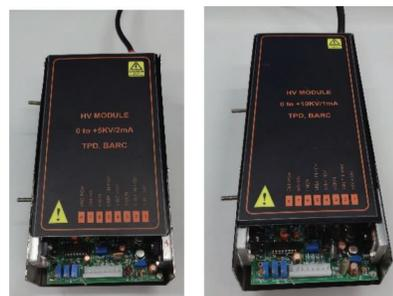
Figure 9. 5kV/2mA and 10kV/1mA HV modules.
