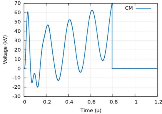
Figure 1. Common mode transient at HV terminals.
