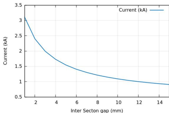
Figure 5. Transient current as a function of inter-section gaps.
