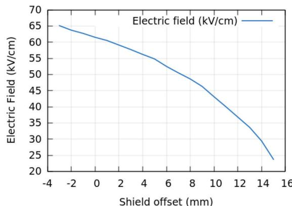
Figure 7. Electric reduction with shield offset.
