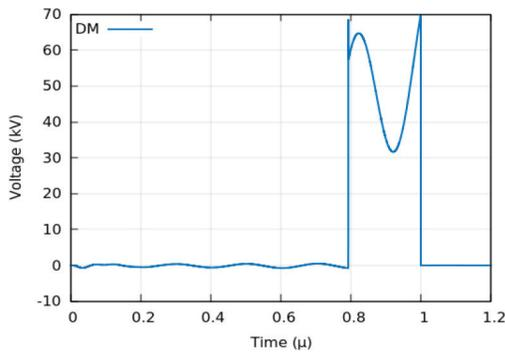
Figure 2. Differential mode voltage across the transformer.
