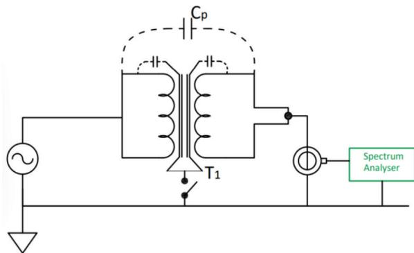
**Figure 8.** Test setup to measure shielding effectiveness.
