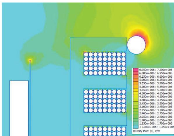
Figure 6. Electric field distribution with a shield.
