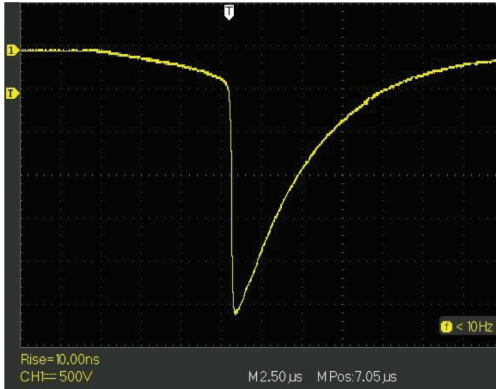
Figure 5. Pulse of RC circuit with thyristor as a switch.
