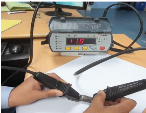
Figure 6. Contact resistance measurement of mechanically crimped lug.
