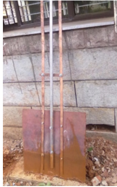
Figure 3. Plate electrode at fabrication stage.
