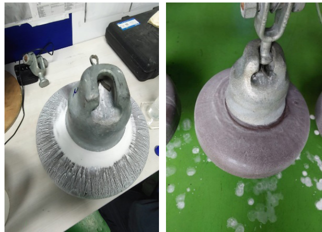
Figure 7. Koalin powder coating on each disc insulator with SDD of 0.1 \text{ mg/cm}^2 .
