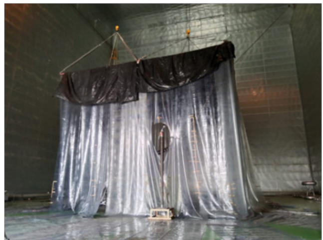
Figure 2. Test chamber for HVDC pollution test.
