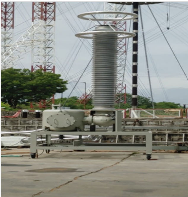
Figure 14. Test chamber for puncture test on DC disc insulators.
