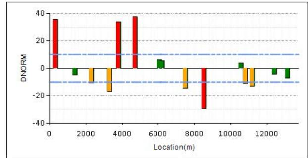
Figure 12. Final DNORM graph quantifying each joint's condition.
