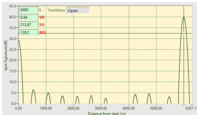
Figure 2. Spot Signature graph of a 6.3 km. cable.
