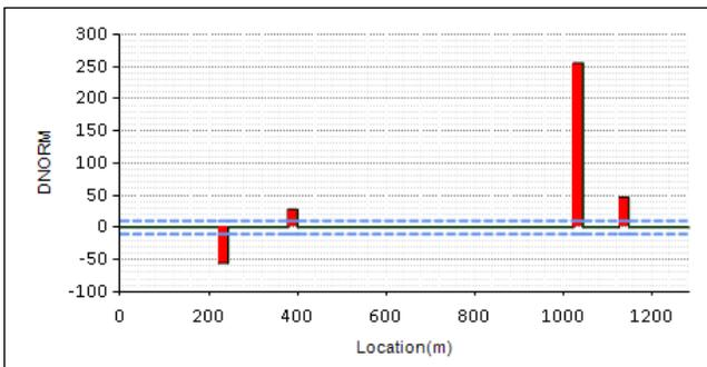
**Figure 14.** Final DNORM graph - after burn-on-arc.
