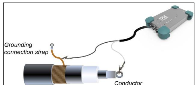
Figure 7. LIRA connection set-up.
