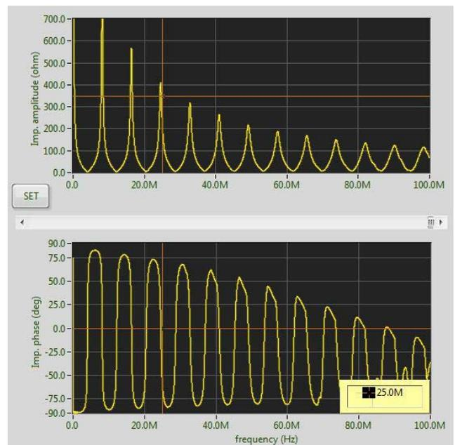
Figure 1. Impedance of an unmatched transmission X line.
