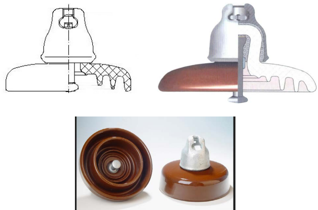
Figure 2. Typical profiles of porcelain disc insulators.
