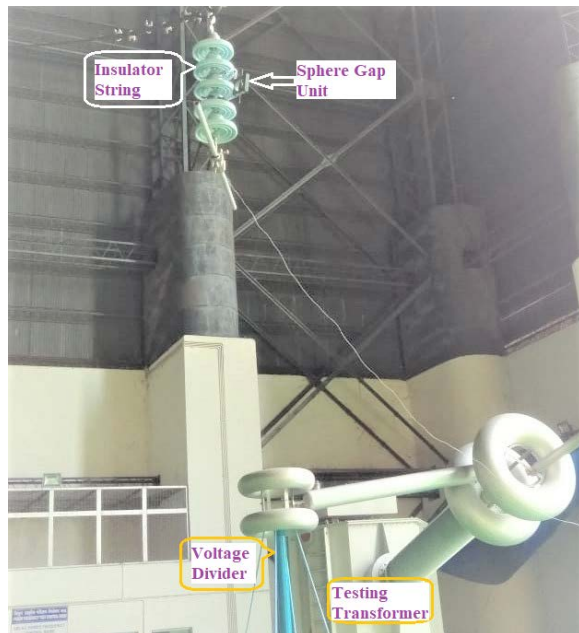
Figure 6. Experimental setup for voltage distribution test.
