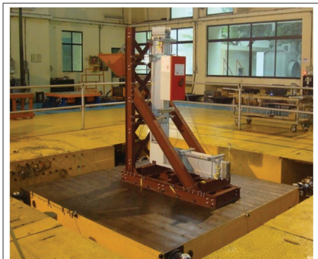
FIG.1 SANDWICH BUSBAR SYSTEM MOUNTED ON SHAKE TABLE
