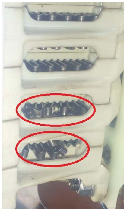
Figure 5. Deformation of transition resistor.
