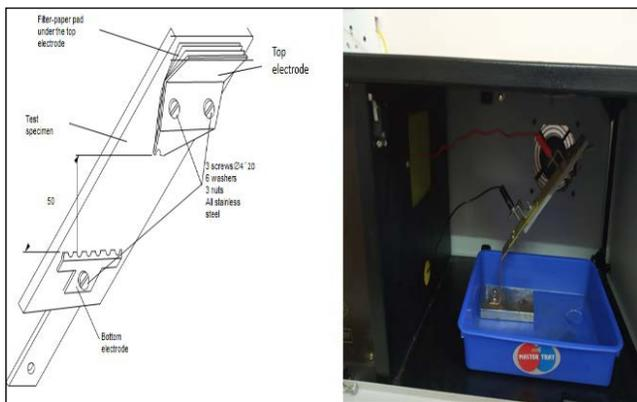
Figure 2. IPTE experimental test set-up.
