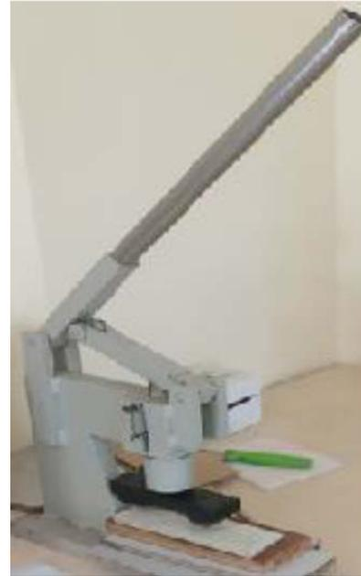
**Figure 8.** Dumbbell cutter press.
