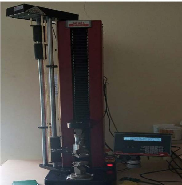
**Figure 7.** Universal testing machine.
