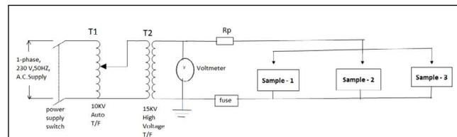
Figure 3. Schematic diagram of corona ageing test.
