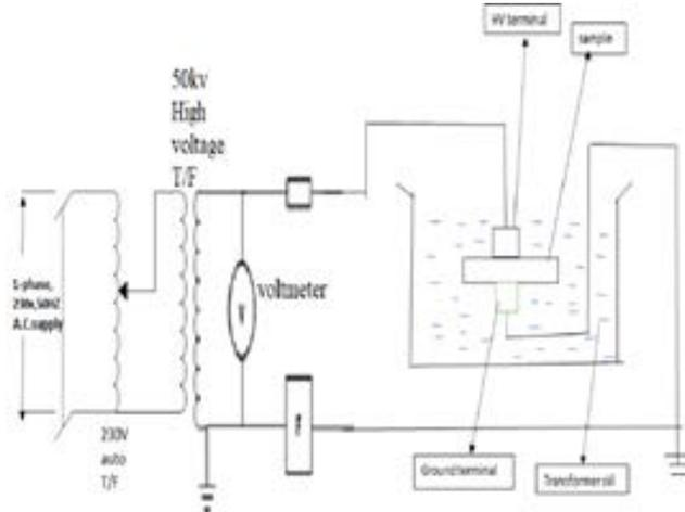
Figure 4. 50kV breakdown voltage tester.
