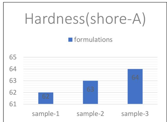
**Figure 19.** Hardness values for different formulations of silicone rubber.
