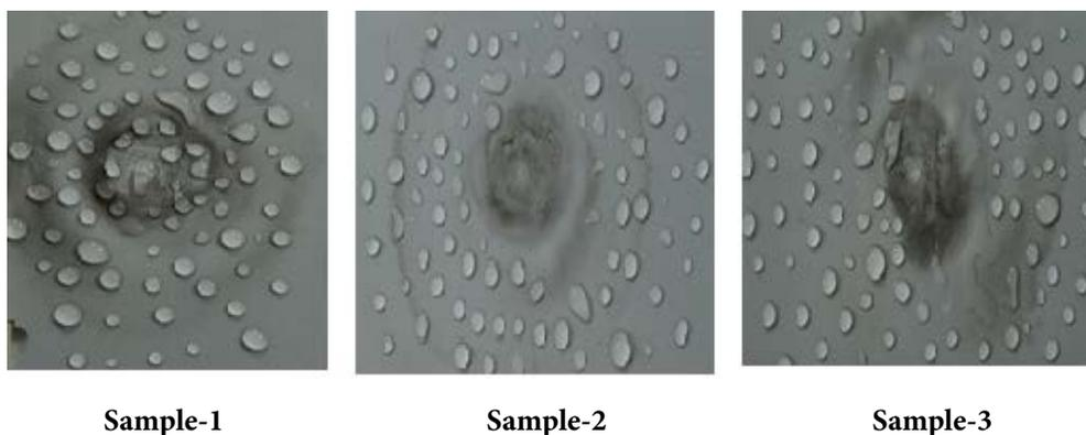
Figure 12. Change of hydrophobicity after the corona ageing test.
