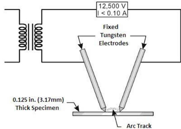
Figure 5. Schematic diagram of arc resistance tester.
