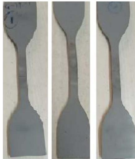
**Figure 9.** Dumbbell-shaped Samples.
