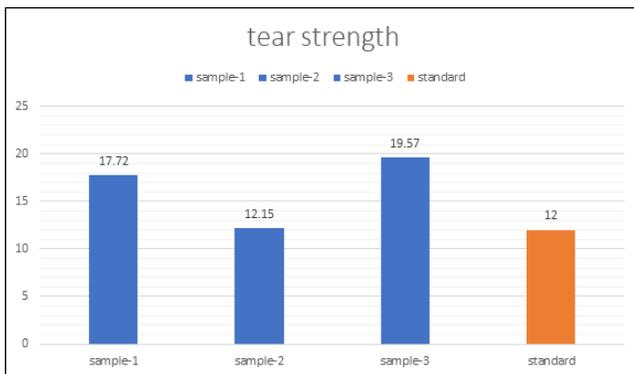
**Figure 18.** Tear strength values for different formulations of silicone rubber.
