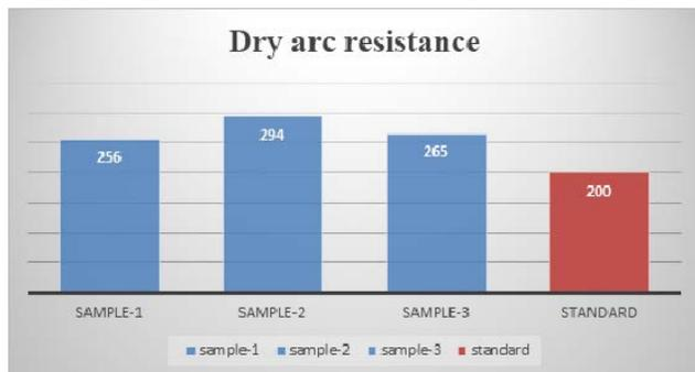
**Figure 15.** Arc resistance values for different formulations of silicone rubber.
