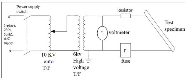
Figure 1. Schematic diagram of IPTE test.
