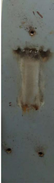
**Figure 20.** Sample after 100 hours IPTE test.
