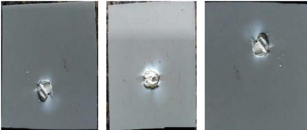
**Figure 14.** Samples after the dry arc resistance test.
