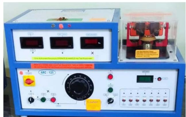
Figure 6. Arc resistance tester.
