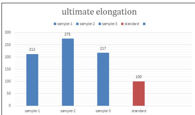
**Figure 17.** Ultimate elongation values for different formulations of silicone rubber.
