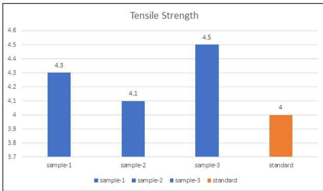
**Figure 16.** Tensile strength values for different formulations of silicone rubber.
