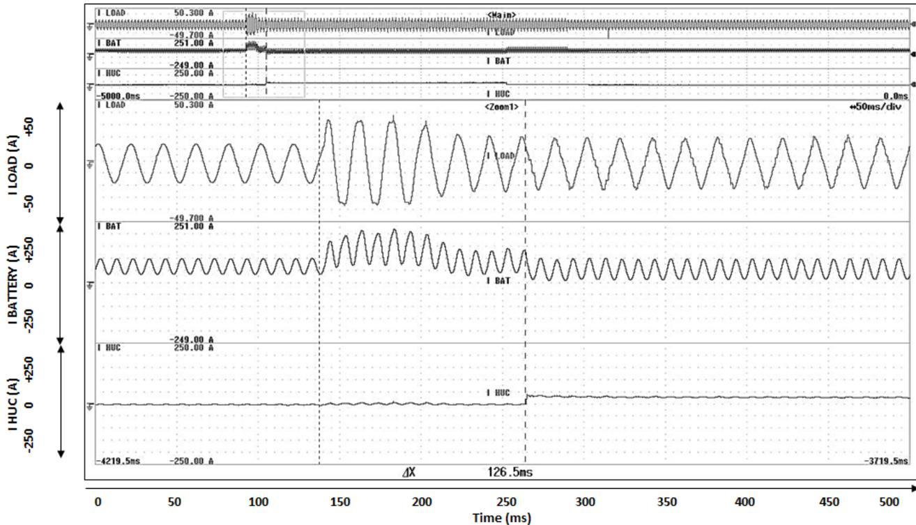
**Figure 7.** Delay analysis from the current profiles
