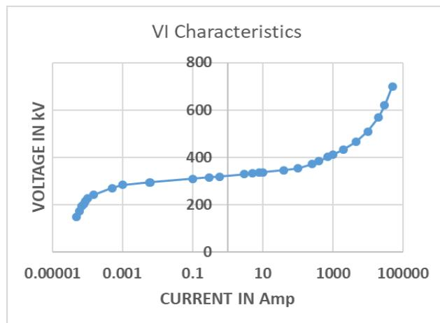
Figure 4. Arrester V-I characteristics.
