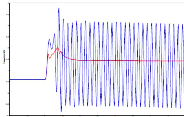
**Figure 7.** Voltage at transformer terminal after the installation of an additional arrester at the transformer terminal.
