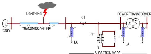
**Figure 1.** Single line diagram of the system considered.
