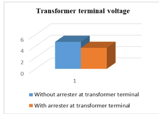
**Figure 8.** Comparison of transformer terminal voltage.
