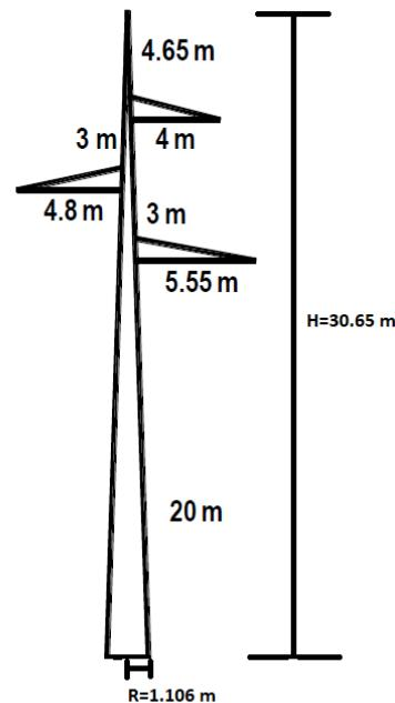
**Figure 2.** Transmission line geometry.
