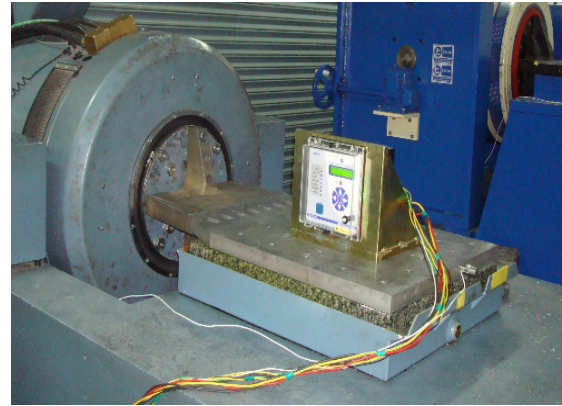
Figure 5. Relay mounted on vibration table
