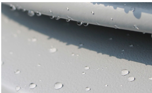
Figure 6. Retained hydrophobicity of Epsilon RTV.
