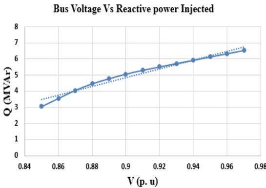
Figure 3. Variation in reactive power compensation for Config 1.
