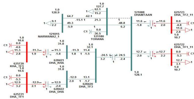
Figure 2. General distribution network configuration for Dhamtaan.
