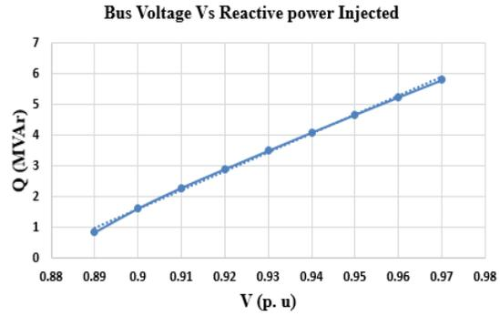
Figure 4. Variation in reactive power compensation for Config 2.
